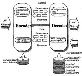
Figure 1: MPEG-4 encoder and decoder architecture.
